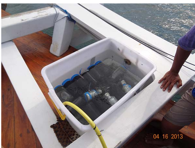
Measurement of primary production under different predefined light conditions – measurement of light intensity.
