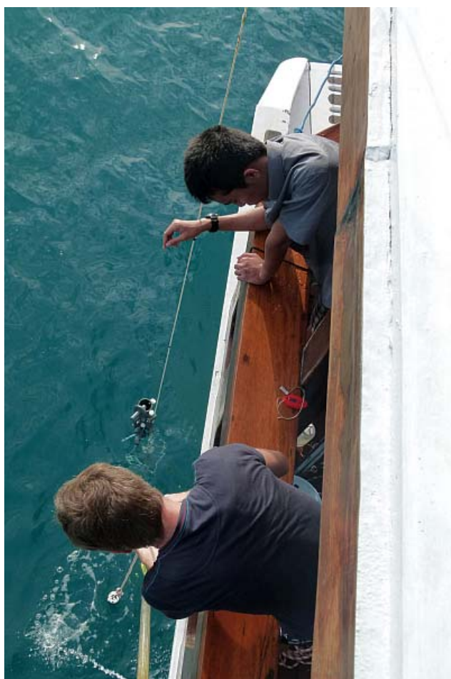
CTD with Niskin bottle for surface water samples and UCTD, a profile from the UCTD.
