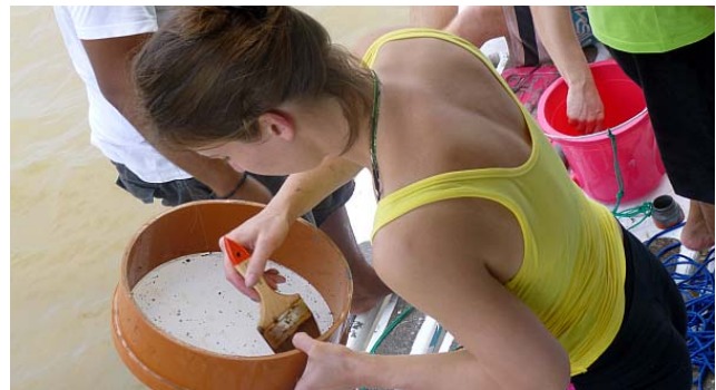
Usage of grab to collect sediment and its passing through a coarse sieve.
