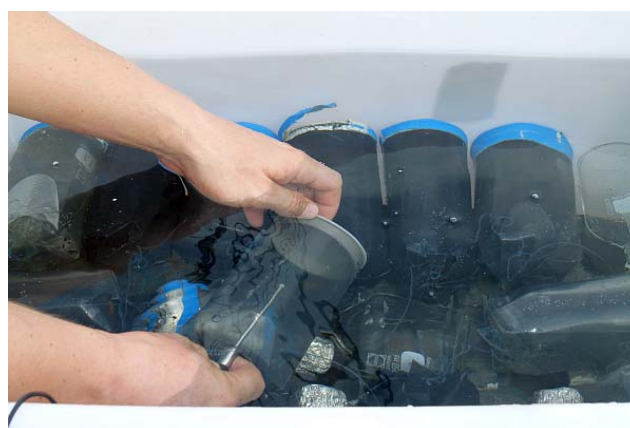
Measurement of primary production under different predefined light conditions – measurement of light intensity.
