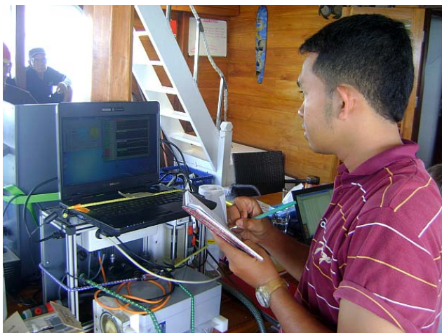
Permanent and underway surface water measurement of pCO 2 , pH, salinity and temperature.
