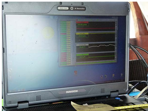
Permanent and underway surface water measurement of pCO 2 , pH, salinity and temperature.
